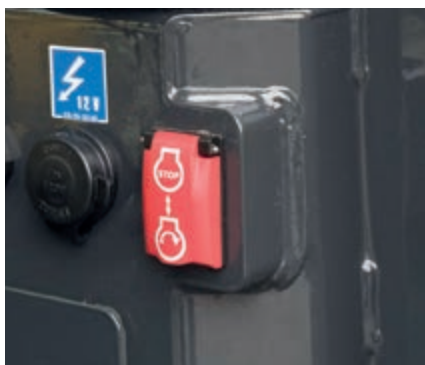
Secondary engine shut down switch
